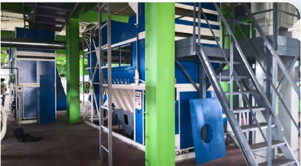
Separators CAD are installed in elevators, feed, seed, grain processing plants and other adapted premises, where the supply of grain to the height of the separator by means of a noria and waste disposal is organized.
