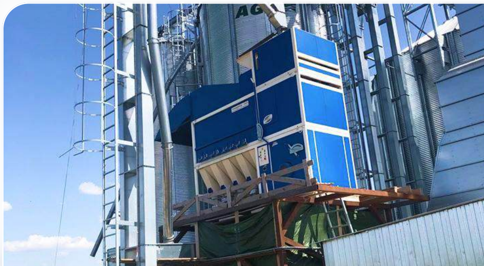
Separators CAD are installed in elevators, feed, seed, grain processing plants and other adapted premises, where the supply of grain to the height of the separator by means of a noria and waste disposal is organized.
